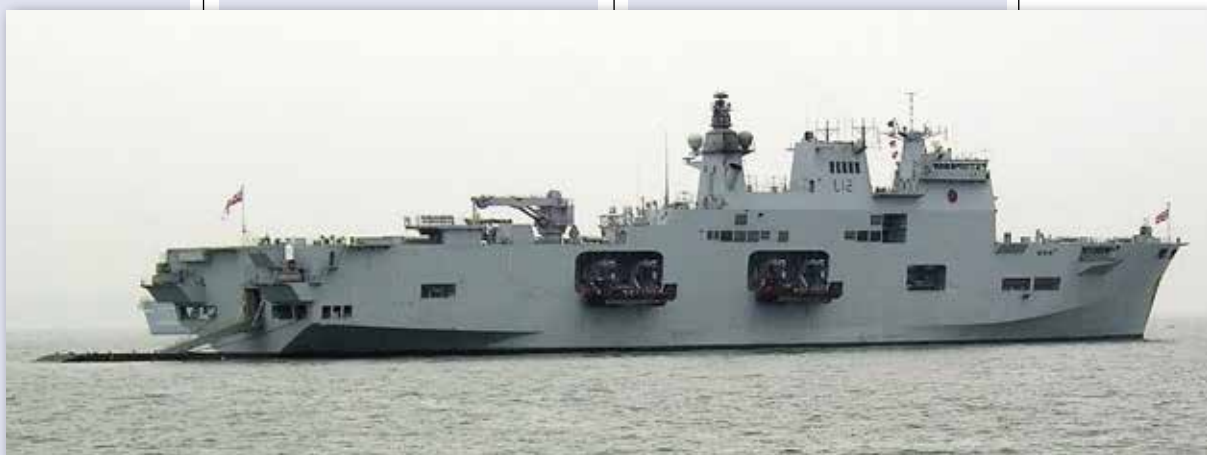
HMS Ocean showing landing craft on davits and stern ramp deployed. (RN)
