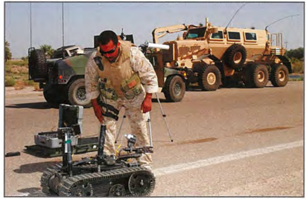
A Marine of the 15th Marine Expeditionary Unit assigned to Explosive Ordnance Team 8 prepares a Talon II remote-controlled robot to go down range and investigate a possible IED along the shoulder of a busy highway in southern Iraq. (Master Sgt. Lek Mateo)
