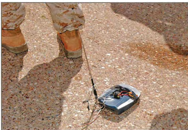
A cordless phone base used as a remote detonating device is recovered by a Marine Explosive Ordnance Team - 8 of the 15th Marine Expeditionary Unit who blew up the IED attached to it. (Master Sgt. Lek Mateo)
