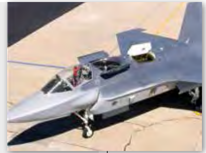
How many are needed? F-35 JSF STOVL with lift-fan open (Defence Industries)
