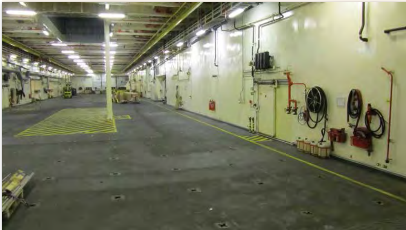
The vehicle deck is approx 1200 linear metres. The total cargo capacity is equivalent to the entire existing RAN amphibious fleet.
