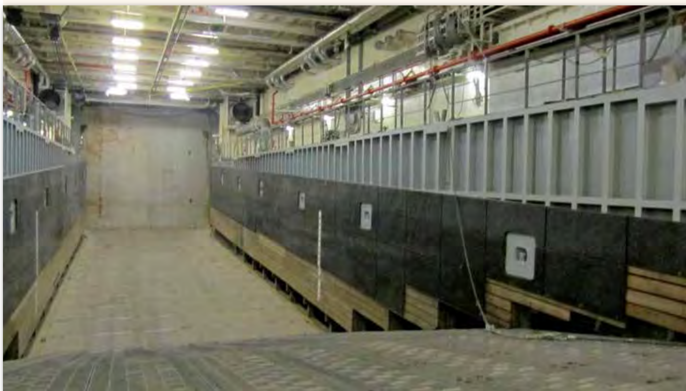
The dock can be flooded and vehicles loaded or unloaded into landing craft directly over the steel beach in the foreground.
