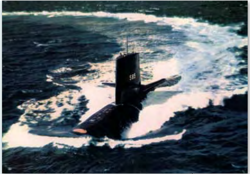
The USS Skipjack was the first nuclear-powered submarine built with the Albacore hull design (USN photo)
