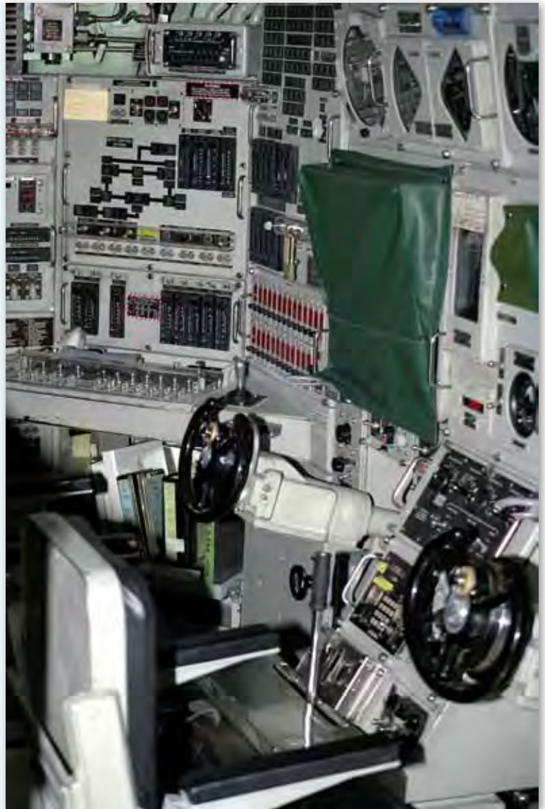
View of the main diving and control station onboard the Los Angeles class nuclear-powered fast attack submarine USS Hartford (USN photo)
