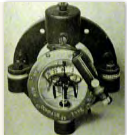
ACO Type 5/17 compass. The horseshoe-shaped structure is the correction mechanism to damp out aircraft magnetic interference known as deviation. This type was used for small machines only. 14
