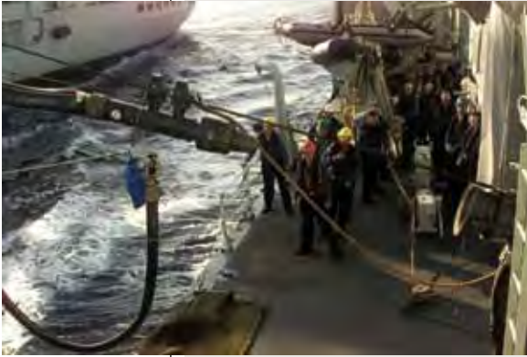
Figure 2: Navy personnel attaching fuelling line during RAS operation (photograph courtesy RAN)
