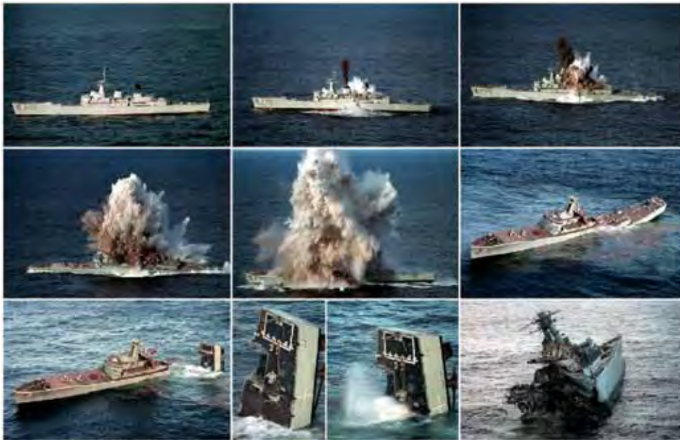
HMAS Torrens under Mark 48 torpedo testing
