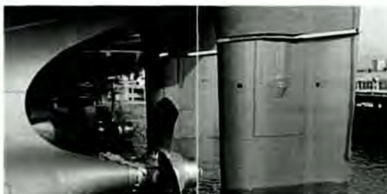
A twin screw, twin Schilling arrangement Source: Hamworthy KSE Ltd
