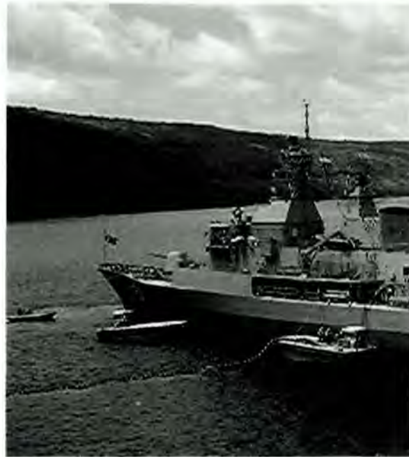
A view from ashore showing the fuelling barge in position with the floating hose visible
