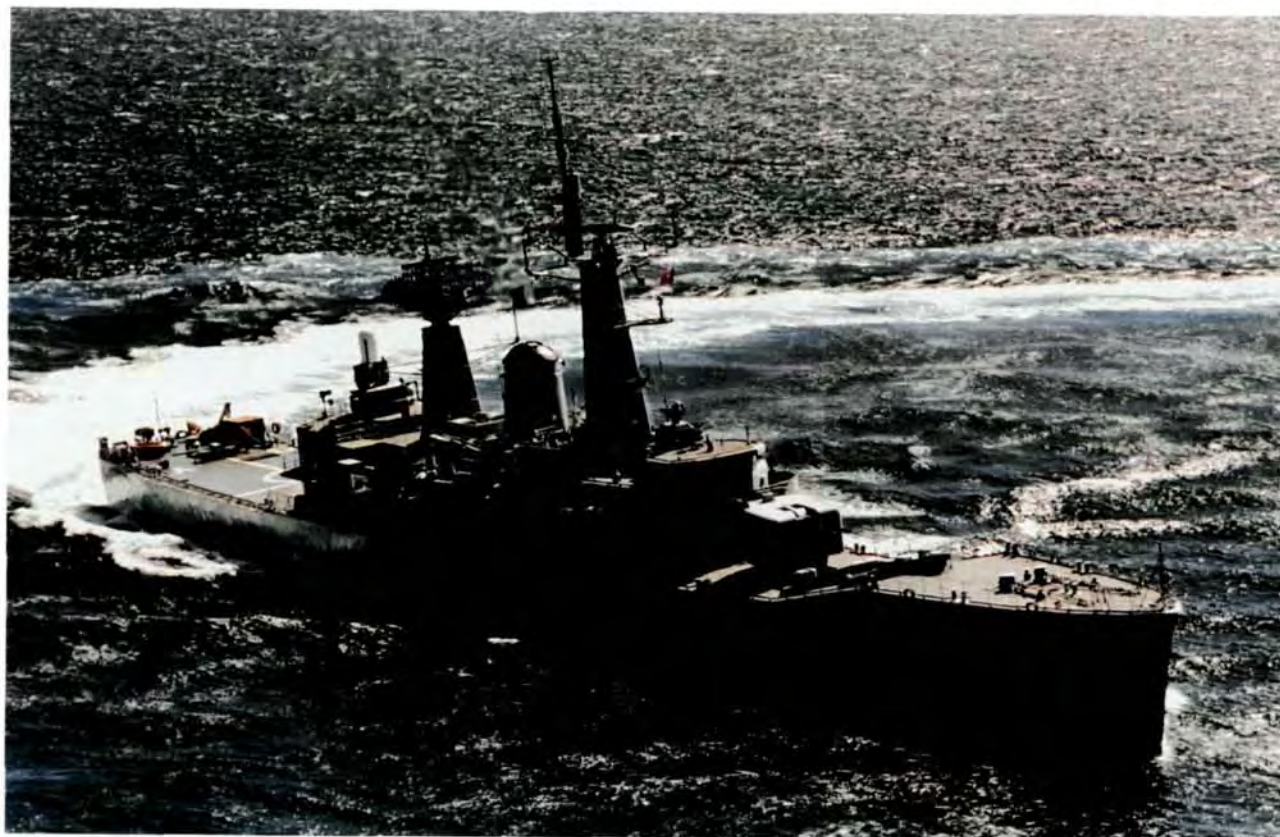
HMNZS Canterbury post refit with CIWS and LWO8 (CMDR Richard Jackson, RNZN)
