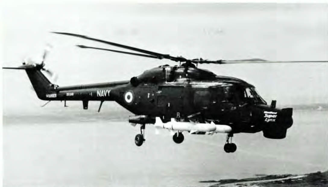
Super Lynx is the latest Westland Navy Lynx, NATTO's standard light ship-borne helicopter. A 'chin-mounted' 360° radar and advanced dipping sonar enable Super Lynx to detect, localise and prosecute targets up to 100 miles from the fleet, operating autonomously in any weather, night and day. Super Lynx has Rolls-Royce Gem 42 engines, a new high-efficiency tail rotor, optional composite swept-tip main rotor blades, and advanced mission avionics based on a central tactical system.
