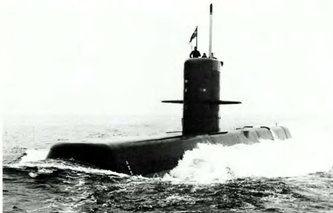
On November 23 the Stirling-Nacken started the sea-trials with its full scale Stirling-AIP system.
