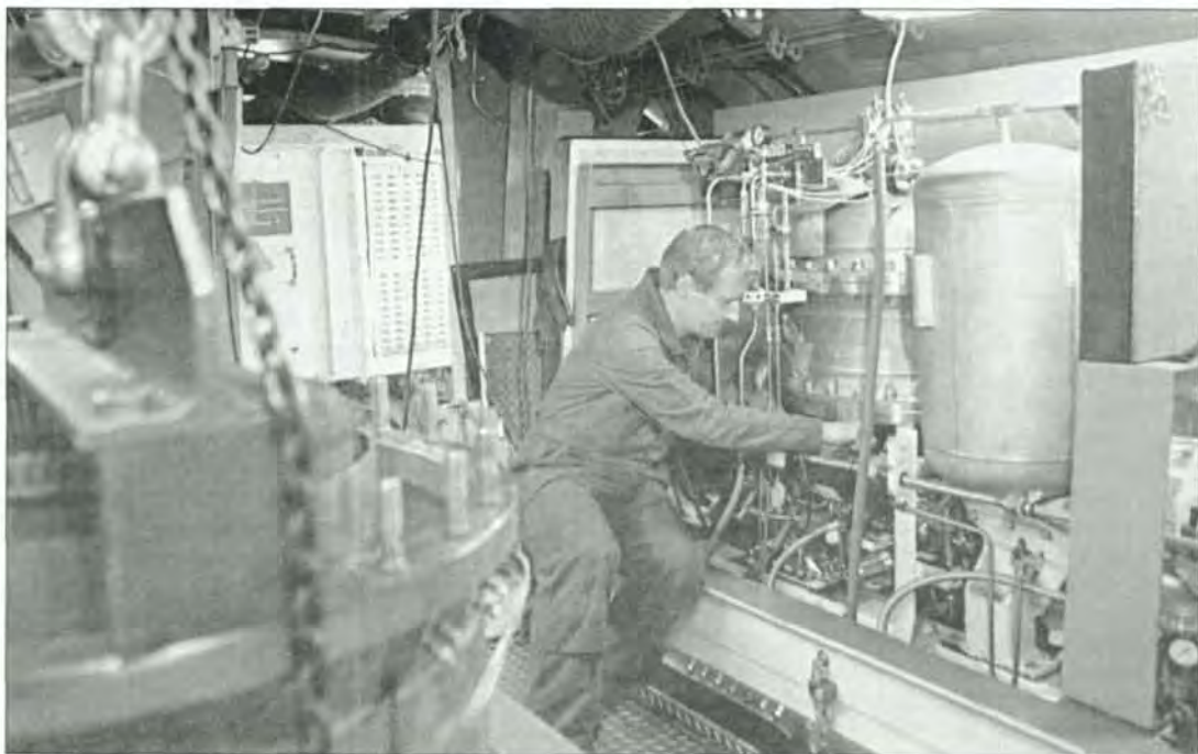
The neutrally buoyant Stirling section is built before the submarine is cut in order to reduce the time the submarine is non-operational.
