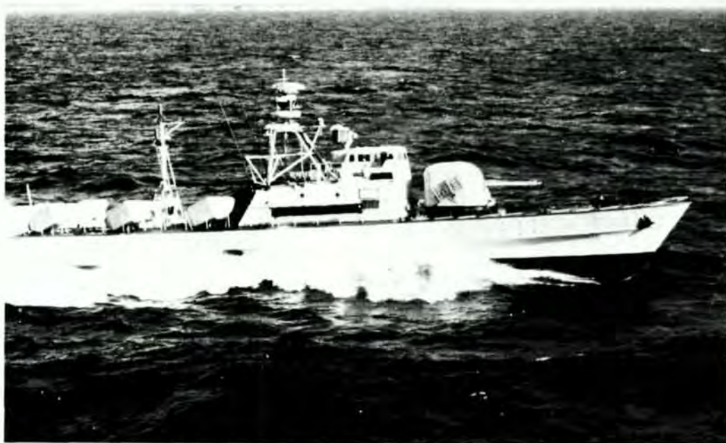
Royal Swedish Navy has taken delivery of Hugin-class patrol boat no. 14 in a series of 16. Length: 36.4 m. Displacement: 150 tons. Speed: 30+ knots. Complement: 18.
