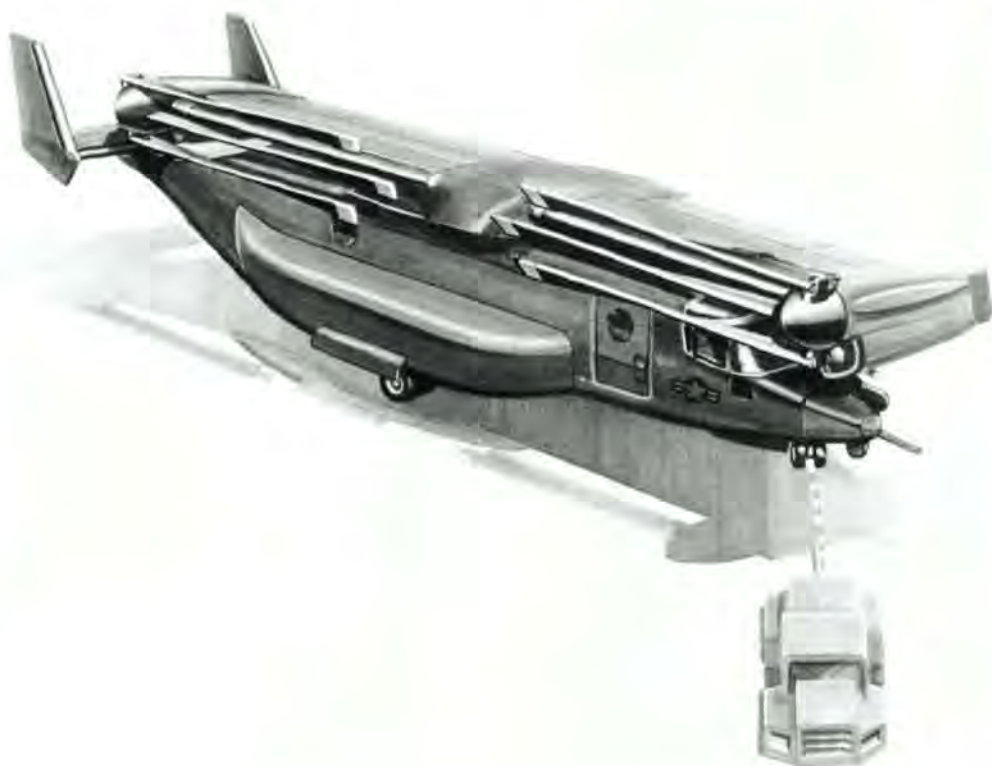
V-22 OSPREY folding arrangements.
