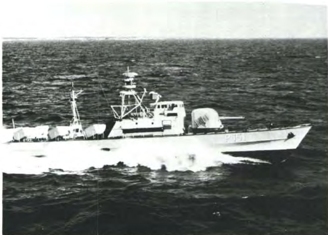
Royal Swedish Navy has taken delivery of Hugin-class patrol boat no. 14 in a series of 16. Length: 36.4 m. Displacement: 150 tons. Speed: 30+ knots. Complement: 18.
