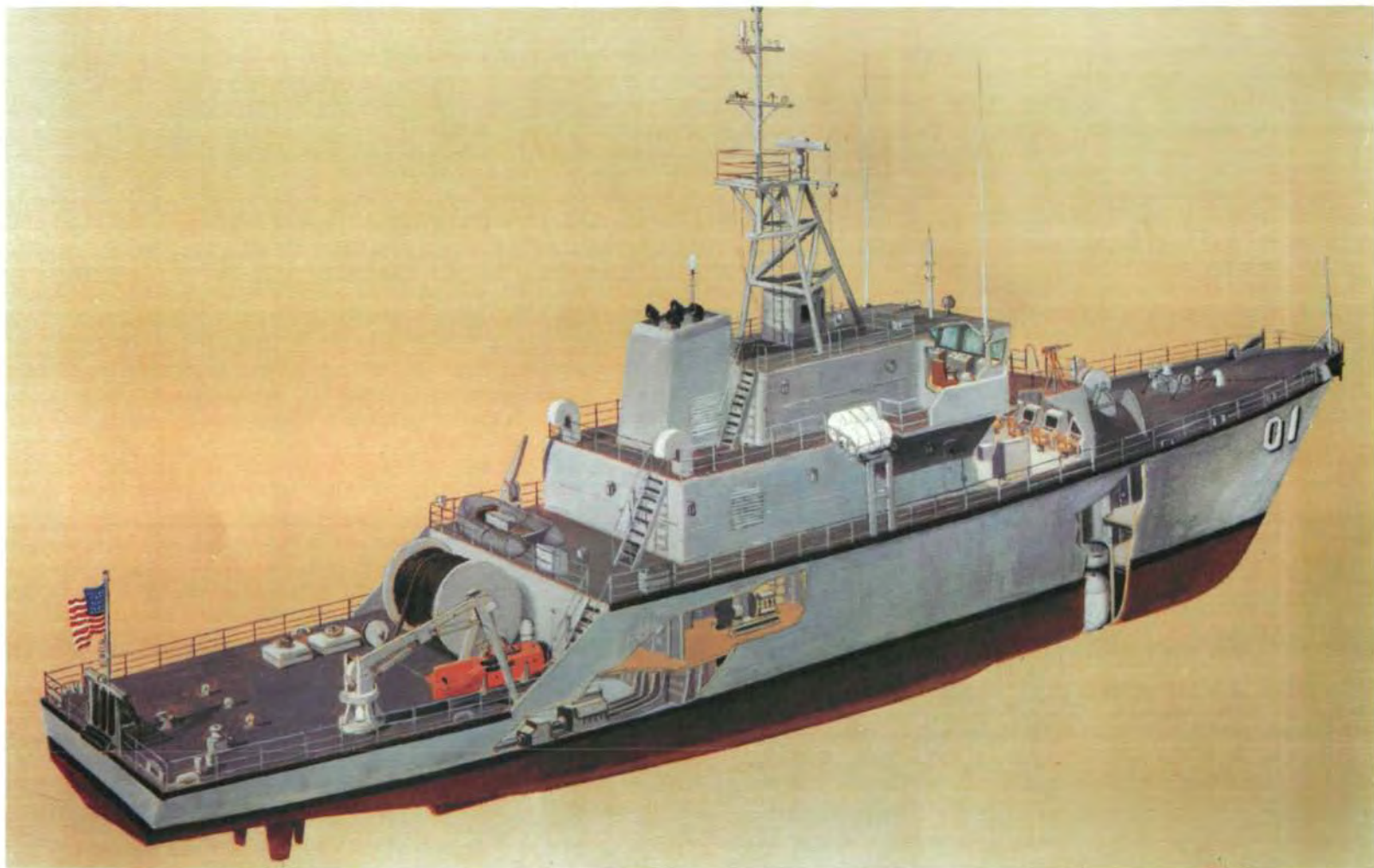
Artist's conception of a minesweeper hunter (MSH) underway. The MSH is a new class of coastal minesweeper that rides on a cushion of air. Courtesy: Official USN Photo
