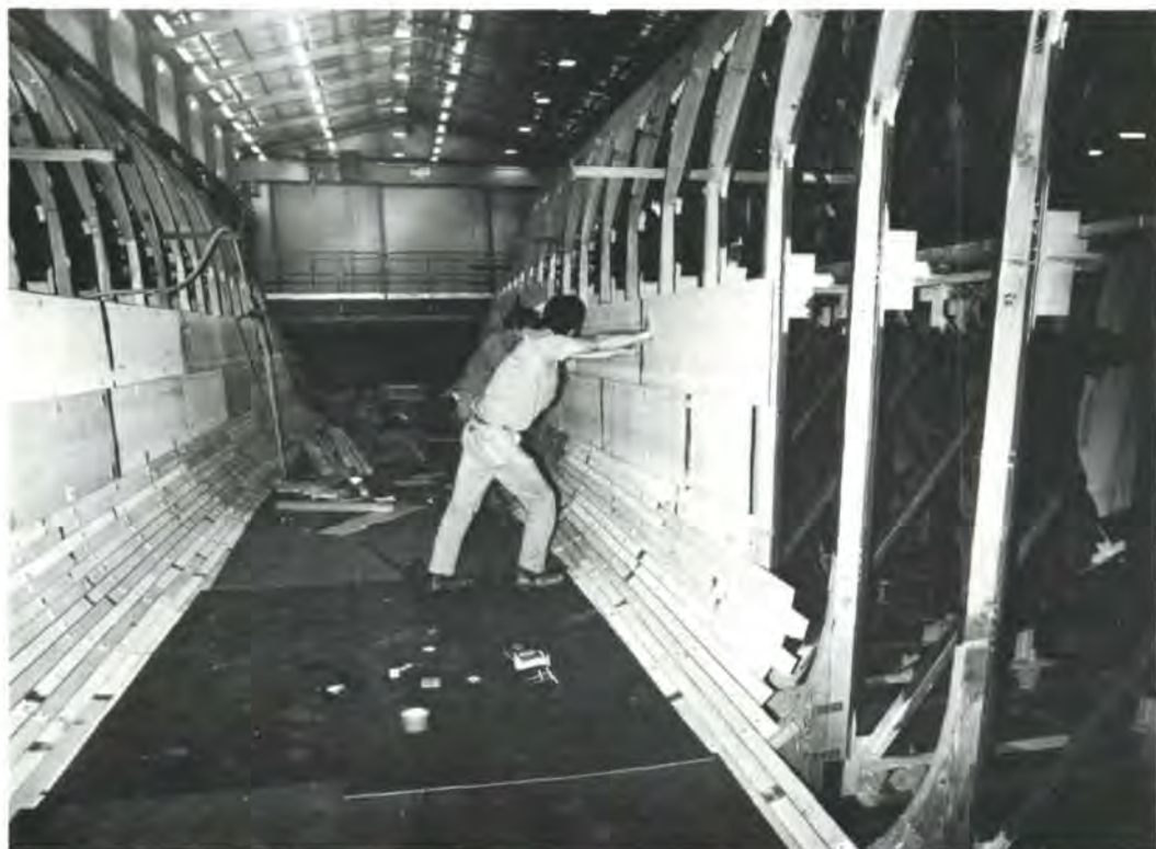
Attaching rigid PVC foam to the inner hull surfaces of the inverted male mould.
