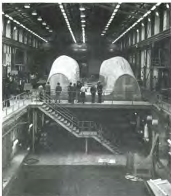
HMAS RUSHCUTTER (MHI 01). Inverted hull prior to fibreglassing.
