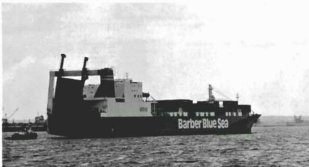
Barbar Tonsberg underway in Baltimore Harbor. This vessel is equipped with bow and stern thrusters. Notice the large stern ramp, the straight lines of her quarter to near the waterline and the bow beginning to cutaway and flare outwardly from amidships.
