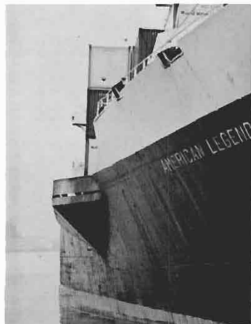
Starboard side profile of American Legend showing her protruding forward knuckle. The ideal position for tug placement would be where this knuckle is located. Tugs must be positioned aft of it losing about 75 feet of leverage. The ship has a similarly designed knuckle aft.
