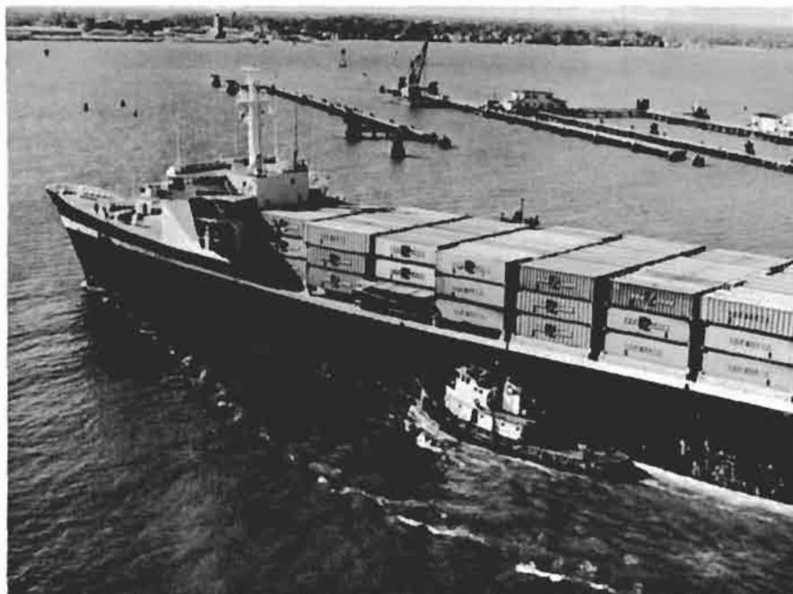
The 948 foot long Sealand Market underway with a tug alongside her port bow. The tug's bow is 150 feet forward the Plimsoll mark or 324 feet after the ship's bow. The ship has recessed bitts but they are below the tug's bow and her head line would jump off the bitts should she use them.
