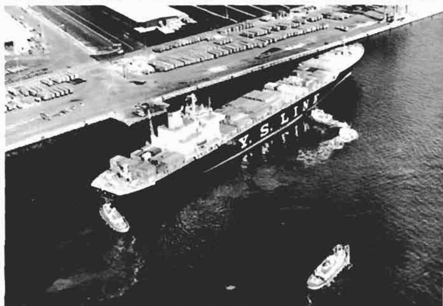
The Tohbe Maru being docked portside to Dundalk Marine Terminal. Notice the after tug can be worked perpendicular across the stern in either direction in lieu of the ship's rudder. The forward tug is only 60 feet forward of amidship making her leverage much less than the lesser powered tug on the stern.
