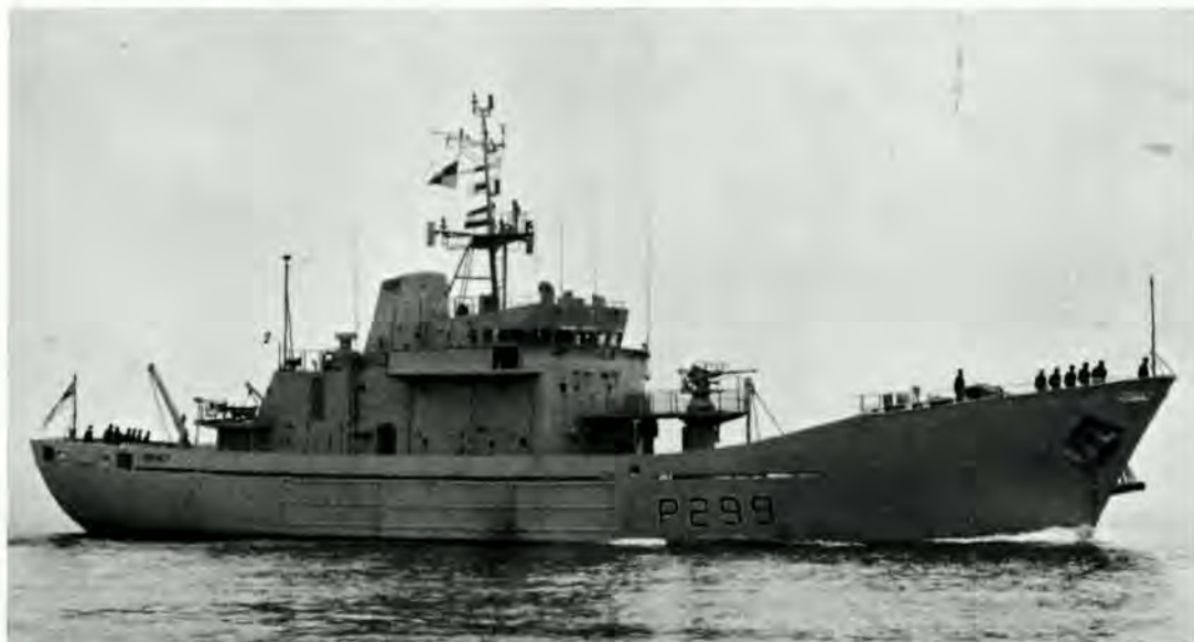
The Island Class patrol vessel HMS ORKNEY (920 tonnes standard displacement, 60 m overall, built 1977, one 40 mm gun, speed 16 knots, complement 34).
