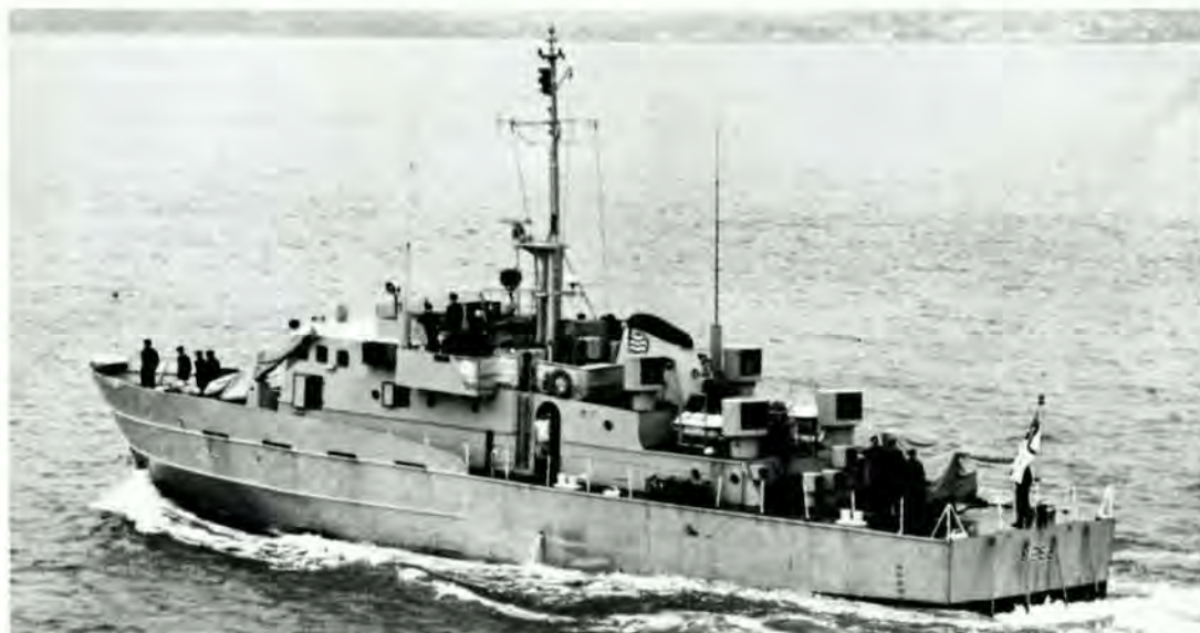
The Bird Class patrol vessel HMS PETEREL (190 tonnes, 37 m overall, built 1977, one 40 mm gun, speed 21 knots complement 24). This class is based on the SEAL Class RAF rescue launches with stabilisers and improved sea-keeping qualities.
