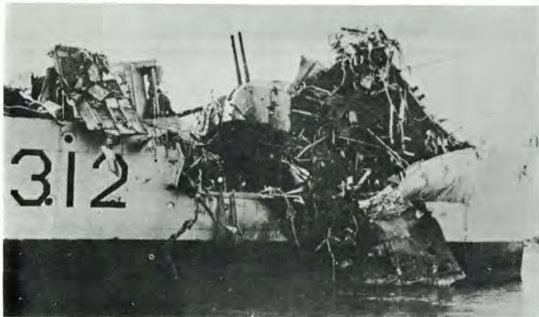
The damage to the Norwegian destroyer, HAUGESUND (formerly the British Hunt class ship, HMS BEAUFORT ), after being hit by a Penguin missile during firing trials in the 1960s.
