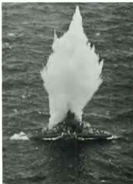
The destroyer escort, USS MOORE , hit by a MK 48 torpedo during weapon lethality trials.
