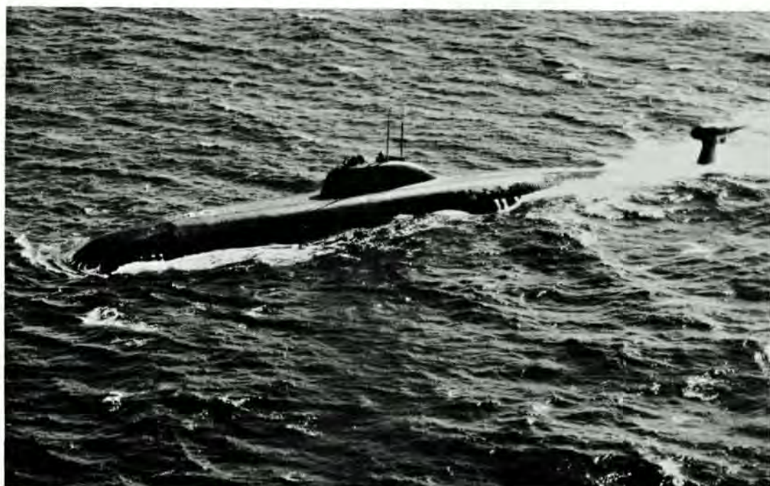
Soviet 'Victor' class fleet submarine. Displacement 3600 tons surface 4200 submerged. Speed 30 plus knots submerged, 26 surface. 8 21 in torpedo tubes. Designed as an attack submarine for both anti-submarine and anti-shipping roles, some Victors are deployed in the Pacific Fleet.
