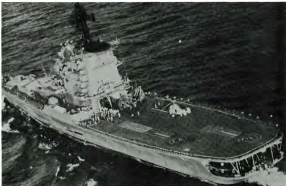
' MOSKVA ' class helicopter cruiser commissioned late 1960s. Displacement 15000 tons standard 18000 full load. Speed 30 knots. Aircraft 18 Hormone A ASW helicopters. Primary role is A/S but has capability for A/A warning, self-defence and a command function.
