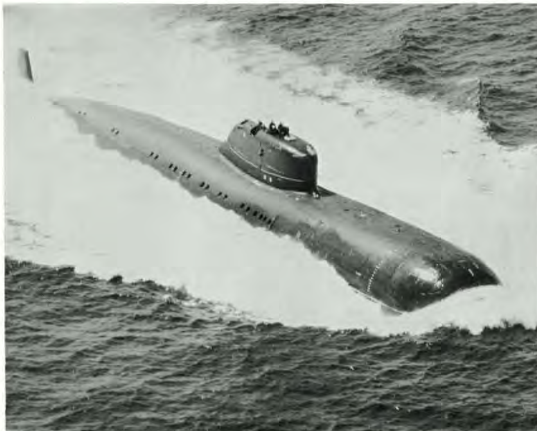
Soviet 'Charlie' class cruise missile submarine (SSGN). Displacement 4300 tons surface, 5100 submerged. Speed 30 knots approximately submerged, 20 surface, 8 missile tubes for SS-N-7 system. Charlies are deployed worldwide for potential anti-carrier battle group operations.
