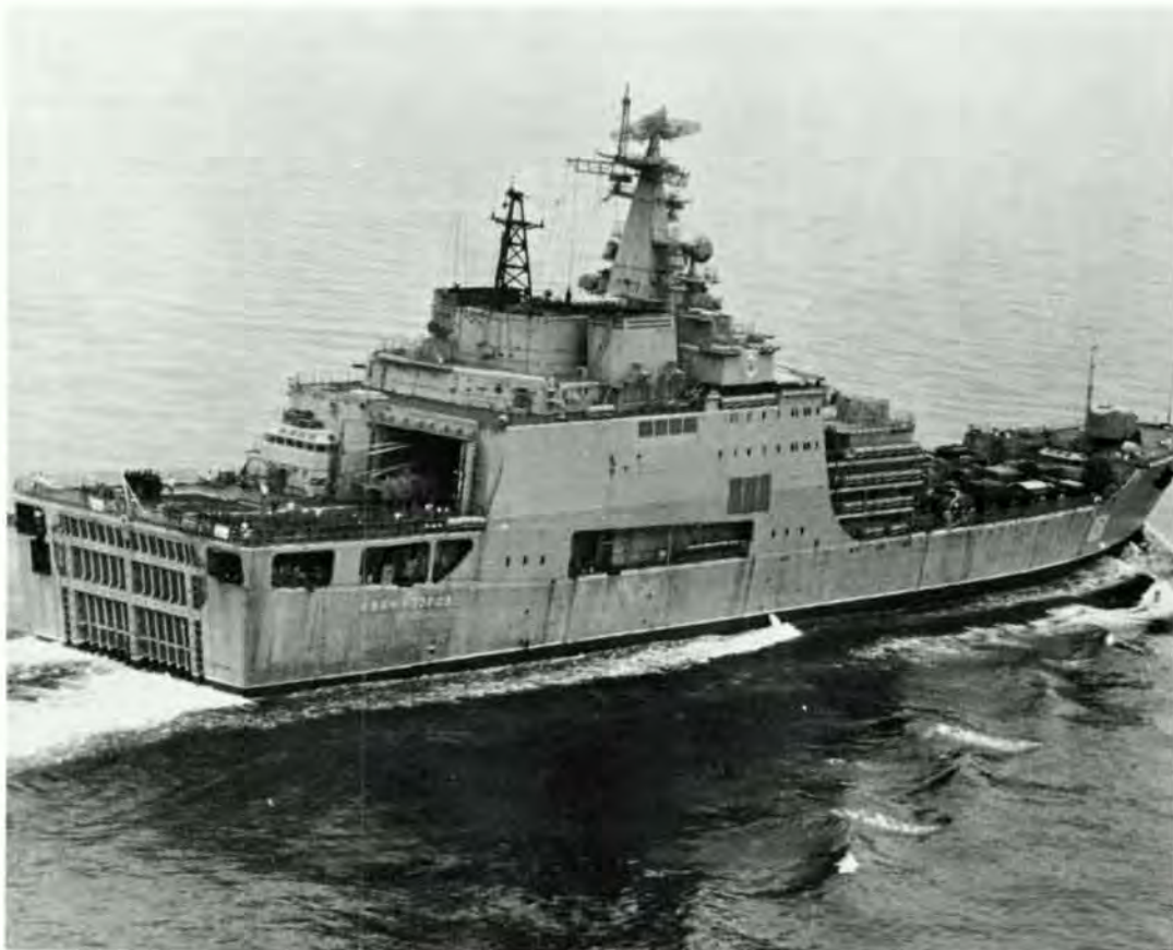
IVAN ROGOV — large amphibious ship (LPD) (11,000 tonnes, 159m overall, 2 76mm guns, 20 knots, and capacity for at least one battalion of naval infantry and up to 40 tanks and other supporting vehicles).
