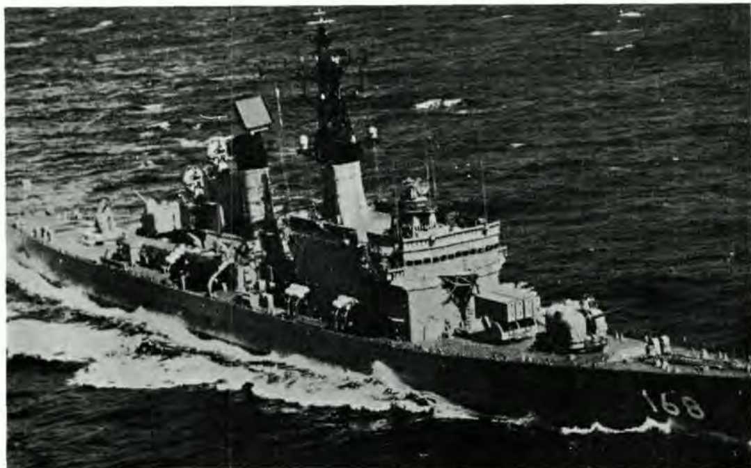
The JMSDF guided missile destroyer TACHIKAZE completed in 1976 (3900 tonnes, 145m overall, standard missile system, two 5in. guns, ASROC, speed 32 knots).
