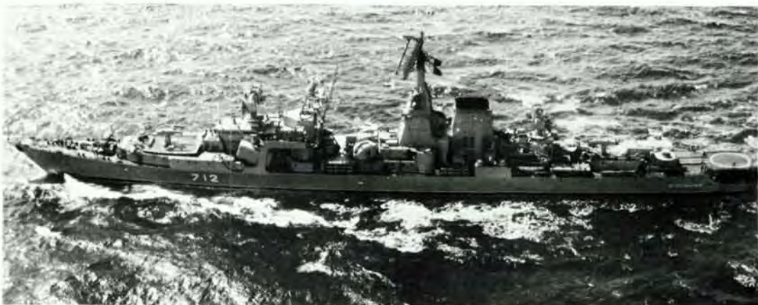
PETROPAVLOSK — KARA Class cruiser (8,200 tonnes, 174m overall, SSN 14, SAN 10, SAN 3 and 4 missile systems, four 76mm guns, 32 knots).
