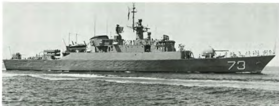
ROSTAM — Frigate built in UK 1972 (1,120 tonnes, 94.5 m overall, Seakiller and Seacat missile systems, one 4.5 in. and two 35 mm guns, one Limbo ASW mortar).
