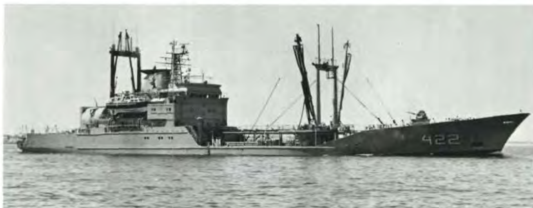
BOOSHEHR — Fleet supply ship built in West Germany 1974 (3,400 tonnes, 108 m overall, one helicopter, combined tanker and store ship).
