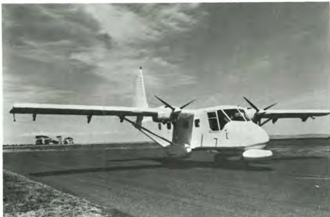
A Nomad Searchmaster variant L aircraft to be used for coastal surveillance in North Australia by the Australian Coastal Surveillance organisation. The Litton 360 0 surveillance radar radome is apparent. Two of these aircraft will be based in Darwin and one in Central Queensland.
