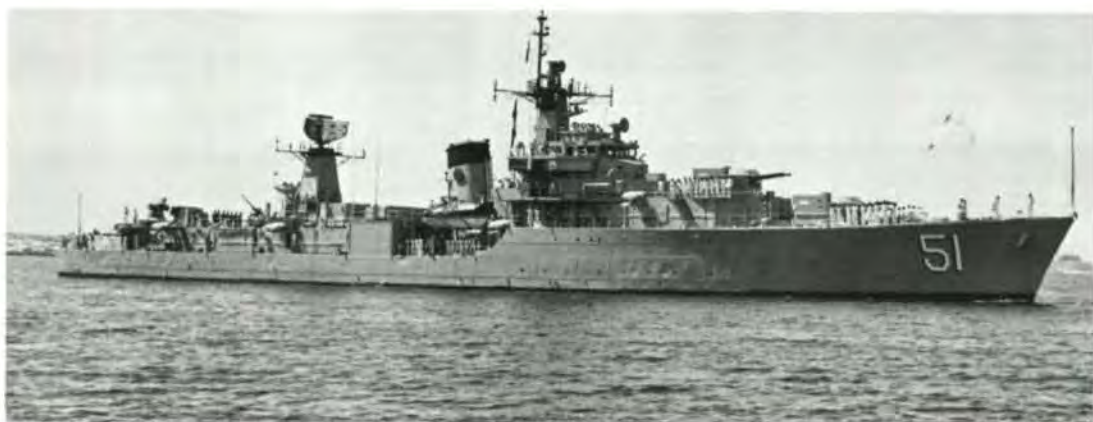
ARTEMIZ —Destroyer built as HMS SLUYS 1946 and transferred to Iran in 1967(2,350 tonnes,108 m overall, four 4.5 in. guns, one Seacat missile system, one squid ASW mortar).
