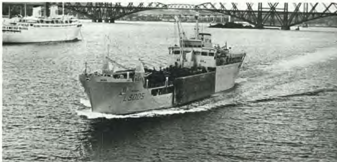
UK LSL SIR GALAHAD leaving Rosyth, Scotland, for a NATO amphibious exercise loaded with vehicles and with MEXEFLOTE pontoons attached to the ship's side.
