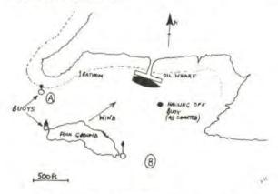
The berthing plan was to pass through Position A, between the foul ground and the point west of the wharf. Although there was a stiff sou'westerly blowing it was well within the ship's capabilities to get alongside and, with a tug to assist, it looked dead easy.
